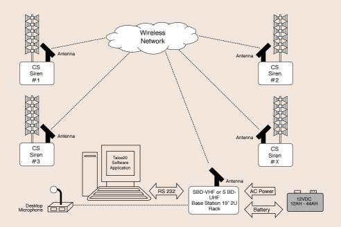
Multi siren system remote controlled by satellite network and computer.
